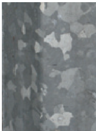
Figure 23.10 The grains of zinc on a galvanised lamp post can be seen clearly
