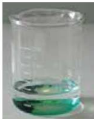
Figure 8.12 The reaction between excess copper(II) oxide and hydrochloric acid to form green copper(II) chloride solution
