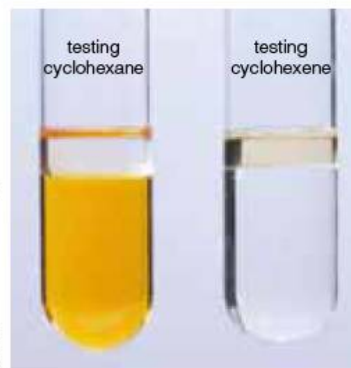
Figure 10.49 The bromine water test for unsaturated hydrocarbons. The unsaturated hydrocarbon decolorizes the bromine water; the saturated compound does not.
