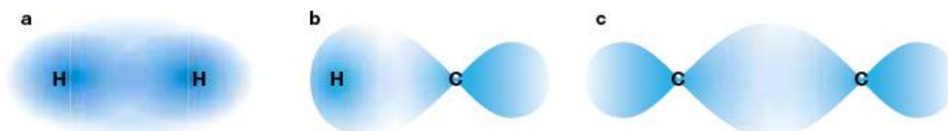
Figure 14.18 Sigma molecular orbitals formed between a hydrogen atoms, b carbon and hydrogen atoms, c carbon atoms
