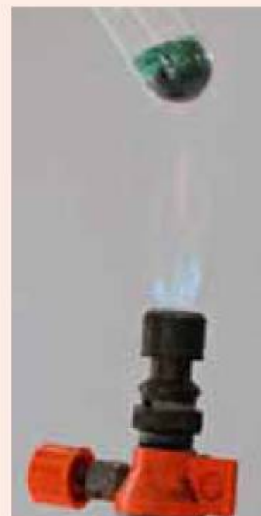
Figure 1.22 Green copper(II) carbonate undergoing thermal decomposition to form black copper(II) oxide and carbon dioxide gas
