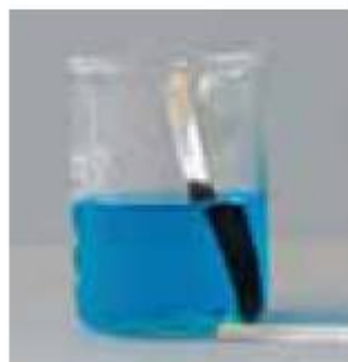
Figure 9.14 The reaction between zinc and copper(II) ions to form zinc ions and copper atoms
