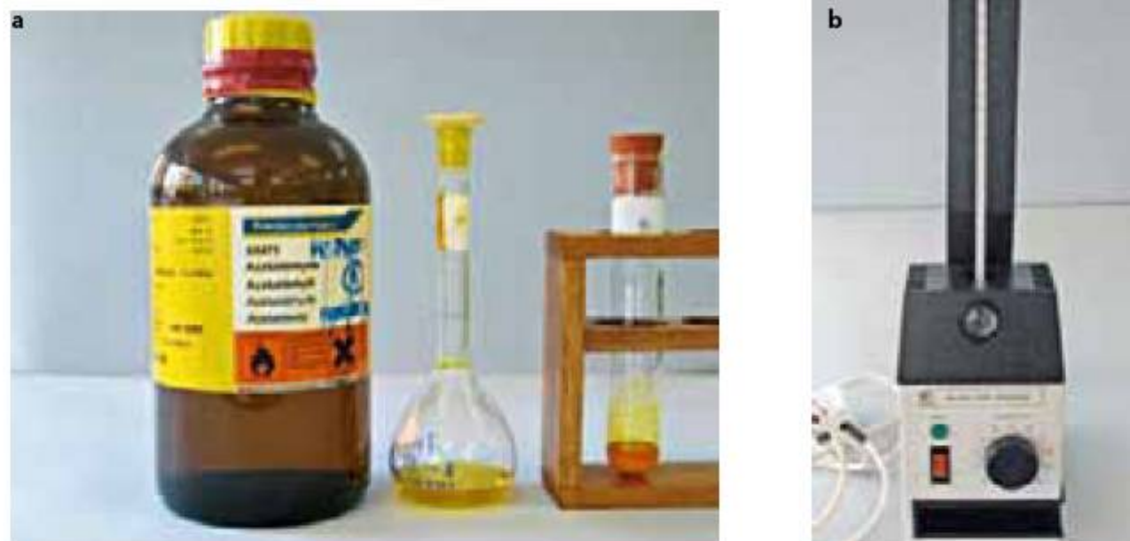
Figure 10.57 a The 2,4-dinitrophenylhydrazine test for aldehydes and ketones. An orange precipitate is formed in either case. b A commercial melting point apparatus
