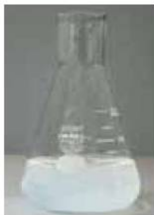
Figure 6.18 The production of a colloidal suspension of sulfur from the reaction between thiosulfate and hydrogen ions
