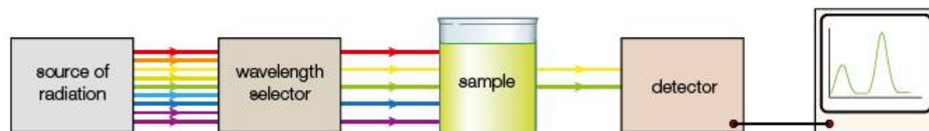
Figure 6.13 Block diagram of a colorimeter or spectrometer
