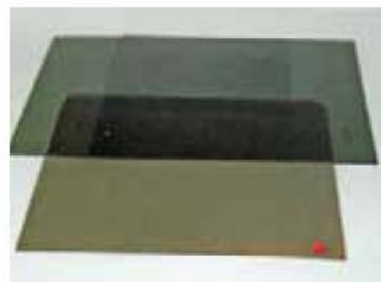
Figure 20.67 If two pieces of Polaroid are laid at right-angles to each other, the light is cut out. This is what is happening at the overlap of the filters here
