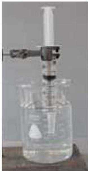
Figure 1.36 A sealed syringe of air in a beaker of hot water
