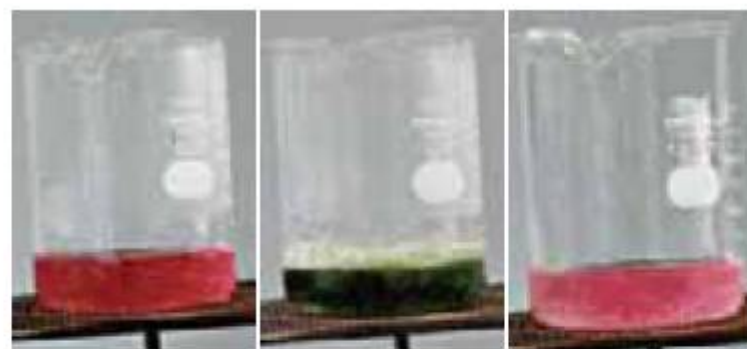
Figure 6.36 The reaction between tartrate ions and hydrogen peroxide in the presence of cobalt(II) ions, acting as a catalyst. The pink solution on the left contains cobalt(II) ions, the green solution in the middle contains a temporary green intermediate containing cobalt(III) ions, and the pink solution on the right contains regenerated cobalt(II) ions
