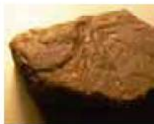
Figure 4.89 An impure sample of corundum: a very hard, crystalline form of the ionic compound aluminium oxide
