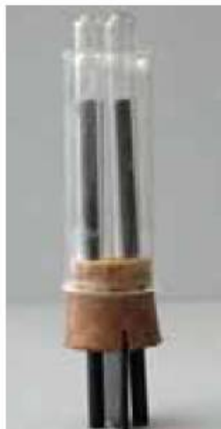
Figure 19.9 Electrolytic cell with graphite electrodes and ignition tubes in which any gases released at the electrodes are collected
