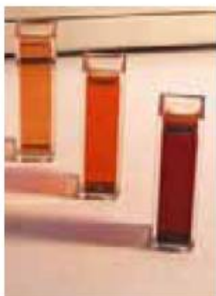
Figure 7.6 The equilibrium between \text{Fe}^{3+}(\text{aq}) ions and \text{SCN}^{-}(\text{aq}) ions can be studied by colorimetry. A soluble blood red coloured complex is formed between the two ions
