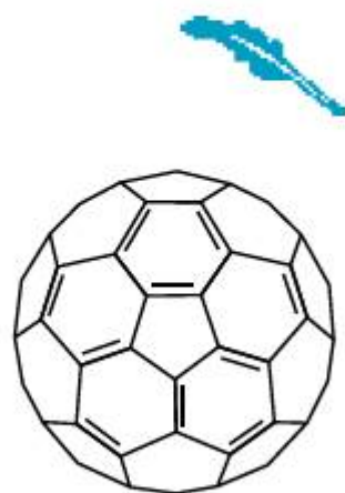
Figure 4.57 The structure of carbon-60 (showing the alternating single and double carbon-carbon bonds)
