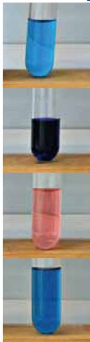
Figure 13.32 Ligand exchange reactions From top to bottom: copper(II) ions, copper(II) ions after addition of concentrated aqueous ammonia, cobalt(II) ions, cobalt(II) ions after the addition of concentrated hydrochloric acid
