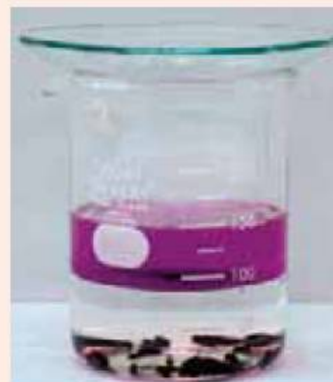
Figure 17.27 Iodine dissolved in a mixture of hexane (upper layer) and water (lower layer)
