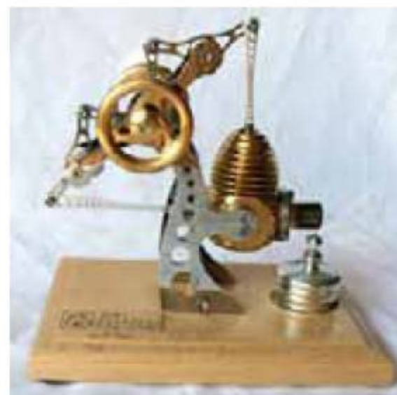
Figure 19.16 A Stirling cycle engine (external combustion engine): the anodized parts are 'gold'
