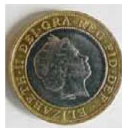
Figure 3.5 British £2 coin showing an outer gold-coloured nickel-brass ring made from 76% copper, 20% zinc and 4% nickel and an inner silver-coloured cupro-nickel disc made from 75% copper and 25% nickel
