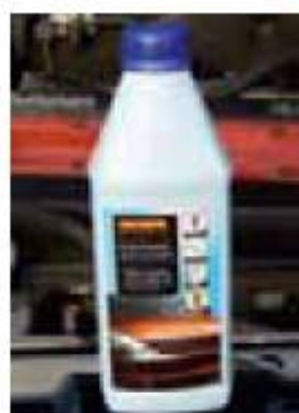
Figure 17.30 A bottle of antifreeze for adding to the water in a car radiator in cold winters
