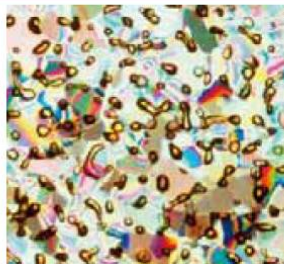
Figure 10.40 Bubbles of methane gas frozen in the polar ice. This is a polarized light micrograph of an ice sample extracted in Antarctica. The sample was from an ice core drilled to a depth of 234m
