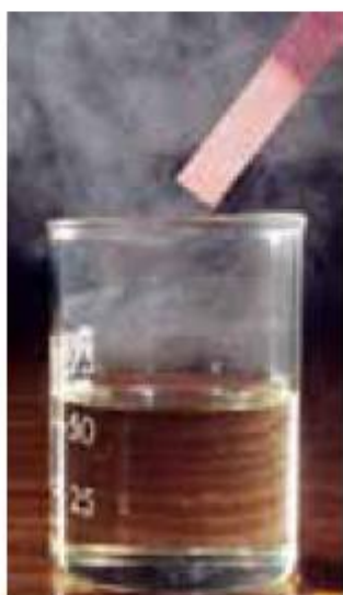
Figure 13.13 The reaction between silicon tetrachloride and water vapour to form acidic fumes of hydrochloric acid that turn blue litmus red
