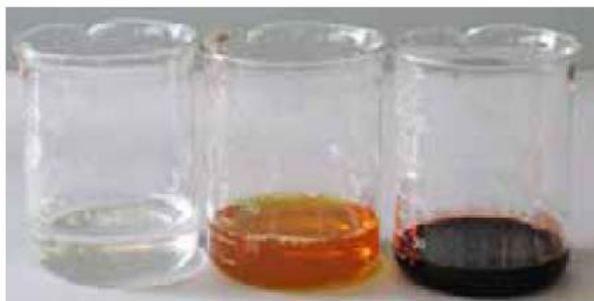
Figure 3.3 From left to right: thiocyanate ions, iron(III) ions and complex ions formed by the reaction between iron(III) and thiocyanate ions
