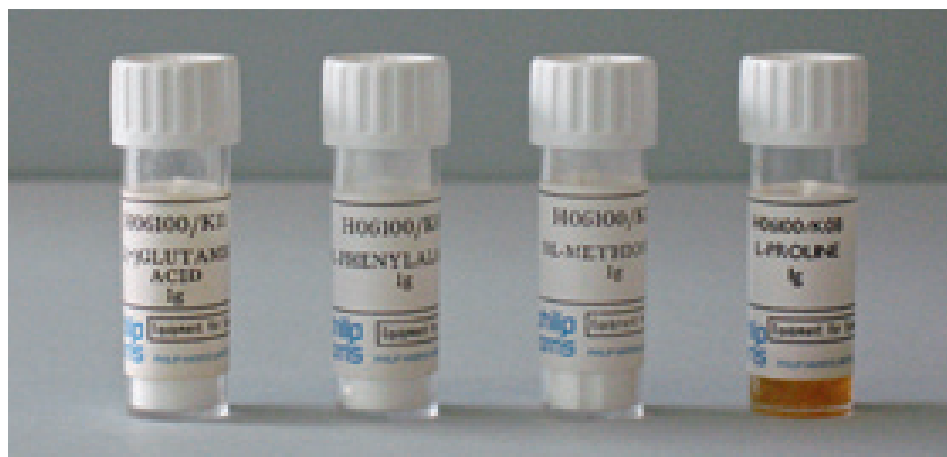
Figure 22.29 Commercial samples of pure amino acids are used as standards during paper chromatography of hydrolysed proteins
