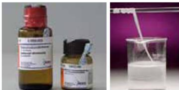
Figure 20.42 a The monomers for the 'nylon rope' experiment (decanedioyl dichloride [or sebacoyl chloride] and 1,6-diaminohexane); b the 'nylon rope' can be continuously drawn off from the interface between the solutions of the two monomers. This experiment produces nylon-6,10
