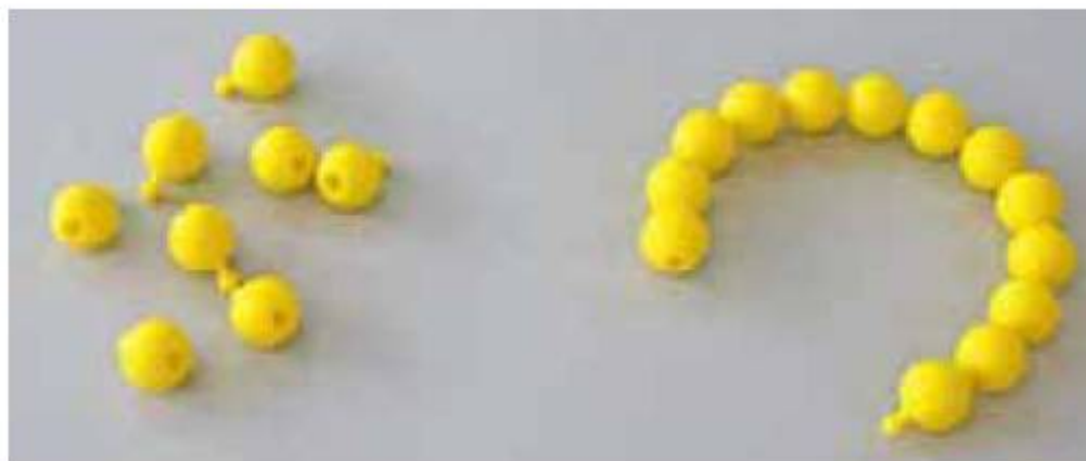
Figure 10.50 The assembly of beads into a chain represents a model of the polymerization process
