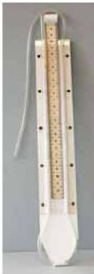
Figure 1.38 Manometer to measure gas pressure
