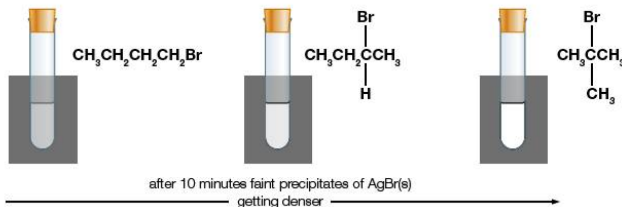
Figure 20.21 The timing of the appearance of the off-white precipitate of silver bromide indicates the rate of substitution of the halogenoalkane
