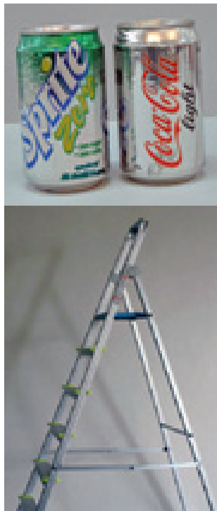
Figure 23.15 Aluminium is light and yet strong; it is also resistant to corrosion.
