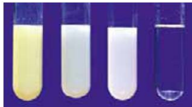
Figure 3.37 The colours of the silver halides – from left to right, silver iodide, silver bromide, silver chloride and silver fluoride
