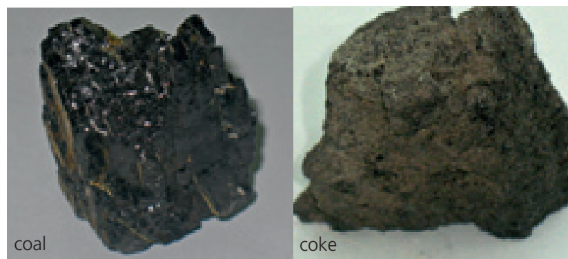
Figure 23.5 A sample of coke – a solid fuel formed by heating coal in the absence of air
