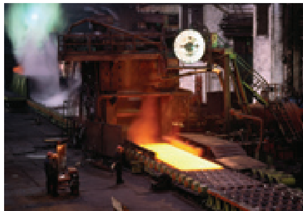
Figure 23.11 A slab of red hot steel being quenched with a spray of cold water – quenching helps to harden the steel
