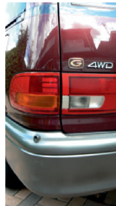
Figure 23.25 Car bumpers can be made of the isotactic form of poly(propene)
