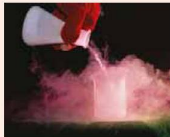
Figure 17.20 Pouring liquid nitrogen that has been separated by fractional distillation of liquid air
