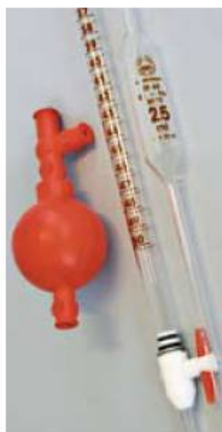
Figure 1.52 A selection of apparatus used in a titration: pipette filler, burette and pipette
