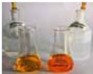
Figure 7.10 The equilibrium between chromate(VI) and dichromate(VI) ions in solution can be manipulated by the addition of acid or alkali
