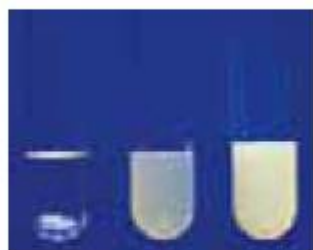
Figure 20.20 Using silver nitrate solution to indicate the release of halide ions during nucleophilic substitution
