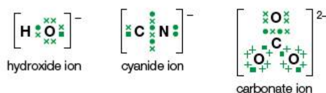
Figure 4.21 Lewis structures (electron dot diagrams) for the hydroxide, cyanide and carbonate ions
