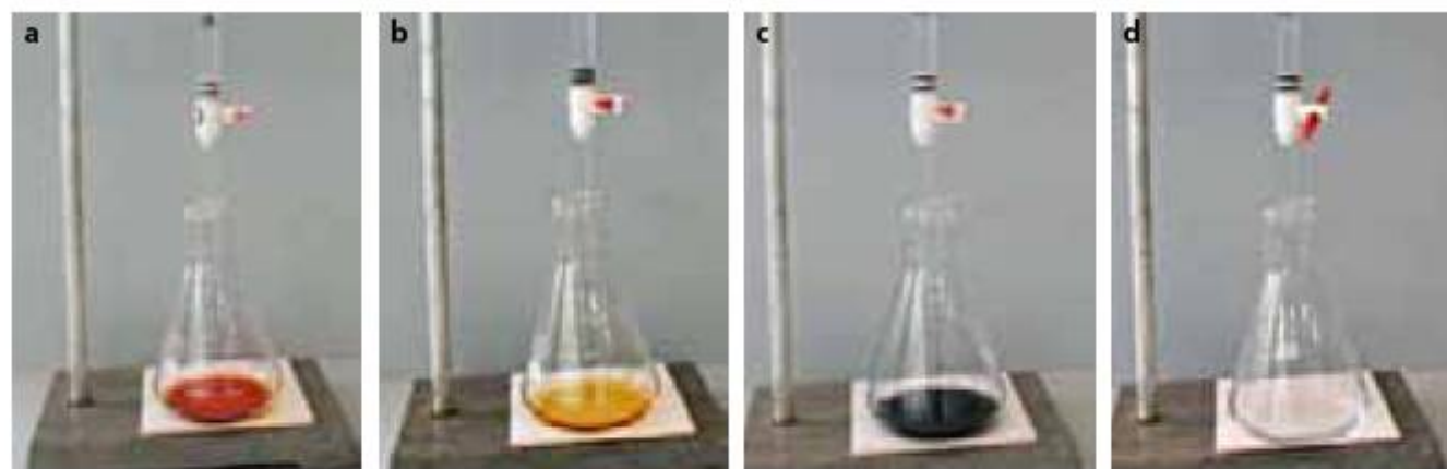
Figure 9.11 The different colours observed during a thiosulfate titration: a aqueous iodine, b addition of the indicator, c deep blue-black colour of indicator with aqueous iodine and d the colourless end-point
