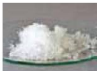
Figure 20.9 Ethanamide is a white crystalline solid at room temperature. The crystals are water soluble because of the capacity of amide molecules to hydrogen bond to water.
