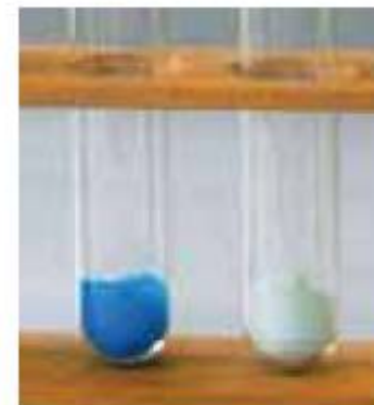
Figure 1.19 Blue hydrated copper(II) sulfate crystals and almost colourless anhydrous copper(II) sulfate crystals
