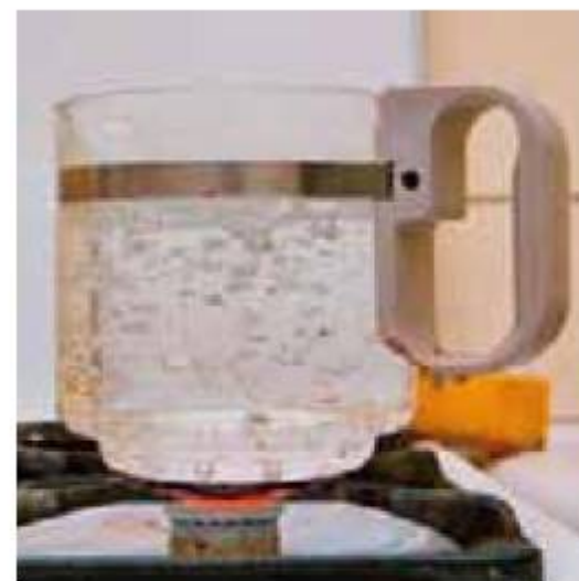
Figure 17.11 Boiling a liquid involves bubbles of gas forming at any point in the liquid, not simply at the surface
